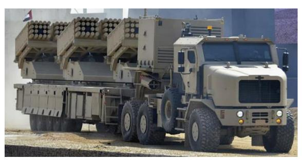
Arabic means Monster with the sensational claim being the world's most **MLRS** powerful system! The Jobaria **MLRS** consists of the American made Oshkosh 6x6 heavy equipment transporter, 10towing
